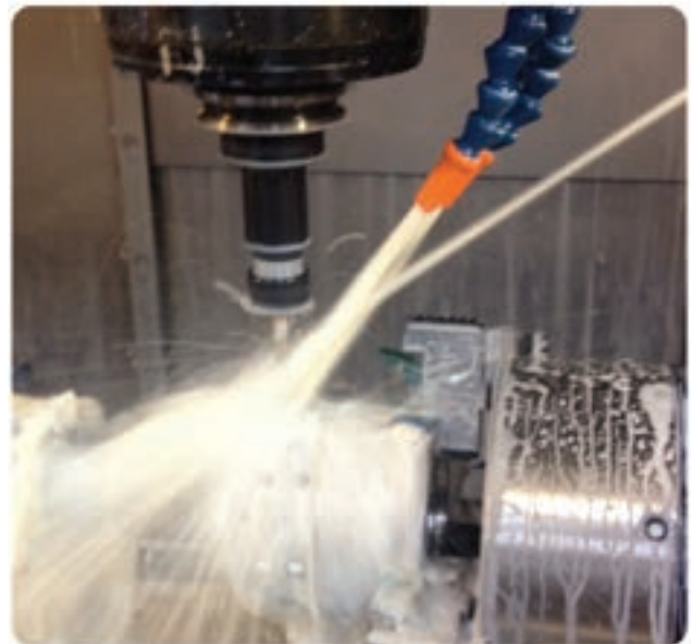
Precision CNC machining of ST-2 Trim
