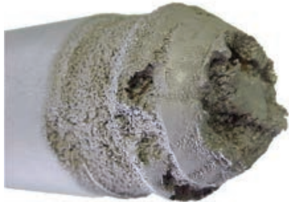
Control Valve Plug Damaged by Cavitation
